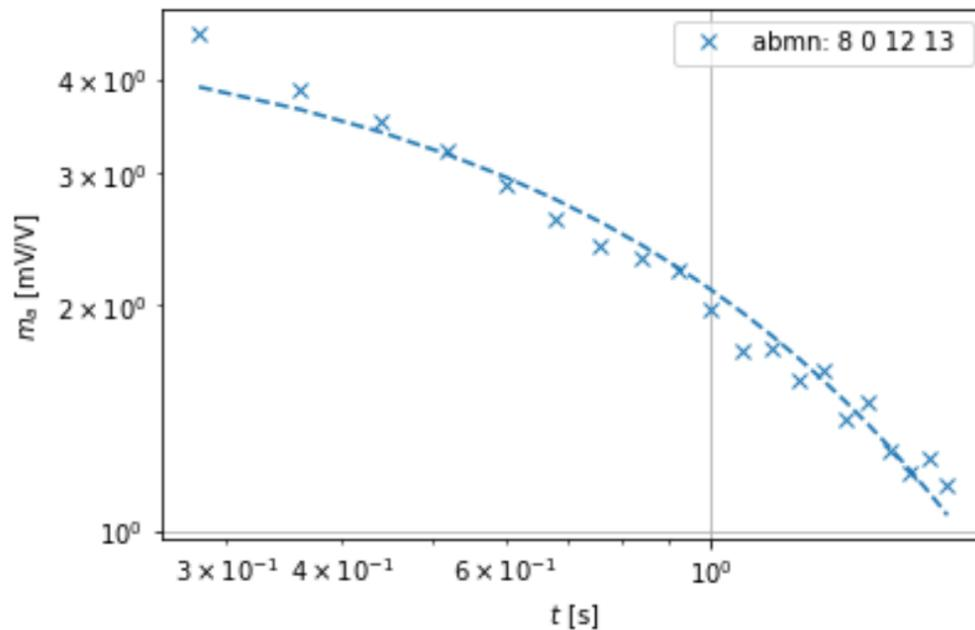
**Figure 6:** the measured IP decay curve (crosses) and the fitted Debye curve (blue dashed).
