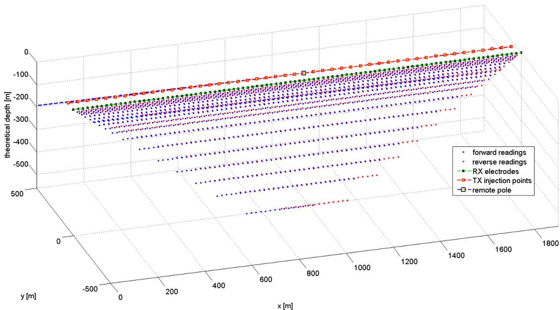
**Figure 15: HIRIP array - Distribution of the data points (TX spacing = 50 m).**
