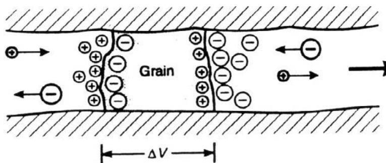
Figure 13: Grain electrode polarization (Reynolds, 1997).
