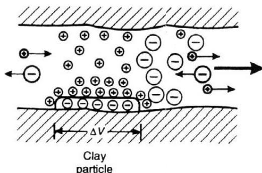
Figure 12: Membrane polarization associated with negatively charged clay particles (Reynolds, 1997).
