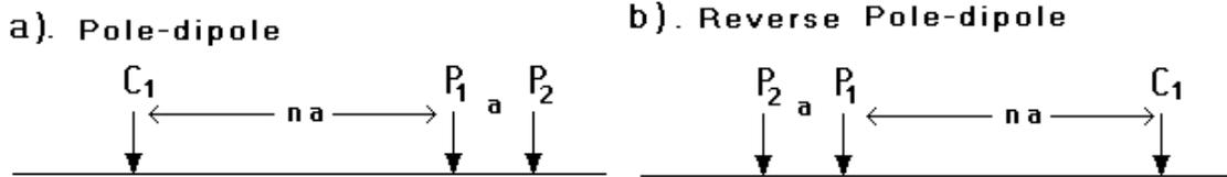
**Figure 14: Pole-Dipole array measured forward (left) and reverse (right) [2-D and 3-D electrical imaging surveys, Dr. M.H.Loke (1996-2004)].**
