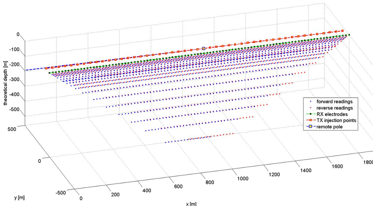
**Figure 1: HIRIP Pole-Dipole array, Data distribution and layout of RX and TX**
