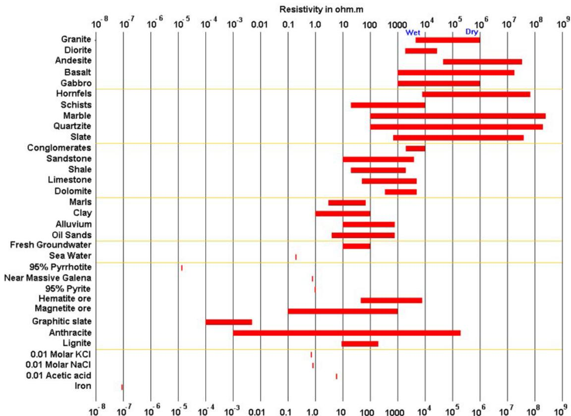
Figure 11: The resistivity of rocks, soils and minerals (M.H.Loke (1996-2001)).
