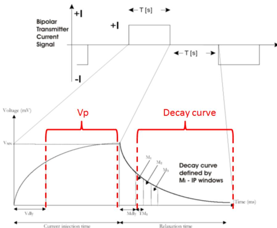
Figure 10: Transmitted current signal and the signal integration.
